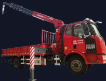
SQ6.3 Truck Mounted Crane (Straight Boom Crane)
